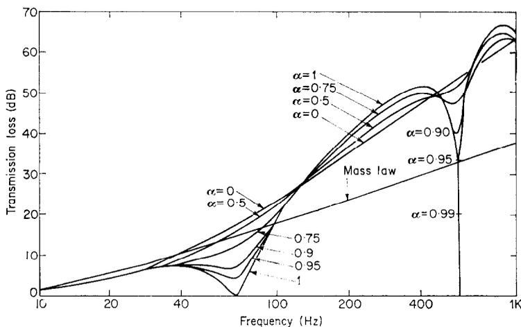
Figure 5. Normal incidence transmission loss, absorbant in cavity.
