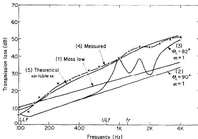
Figure 3. Transmission loss of double aluminium panel.
