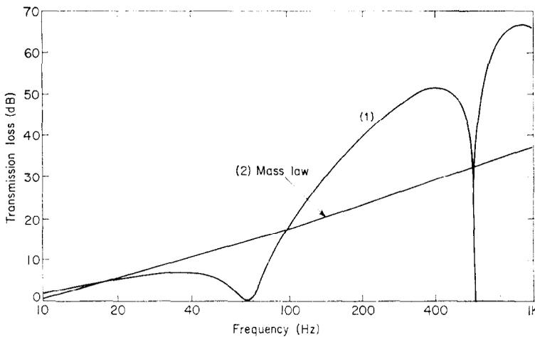
Figure 2. Normal incidence double panel transmission loss  $m = 0.5 \text{ g/cm}^2$ ,  $L = 1 \text{ ft}$ .
