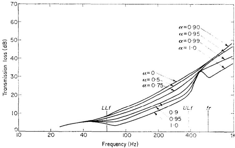
Figure 6. Random incidence transmission loss, absorbant in cavity.
