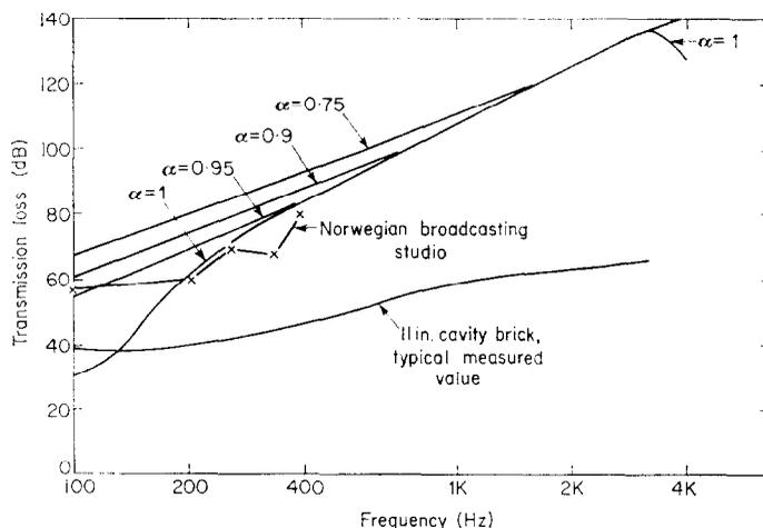
Figure 7. Transmission loss of double brick wall.
