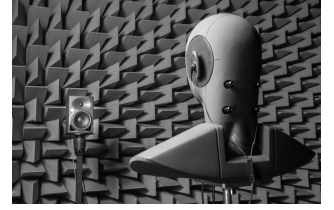
FIGURE 7: Horizontal plane measurement with Neumann KH120 loudspeaker for enhanced low frequency range (1.5 m distance).
