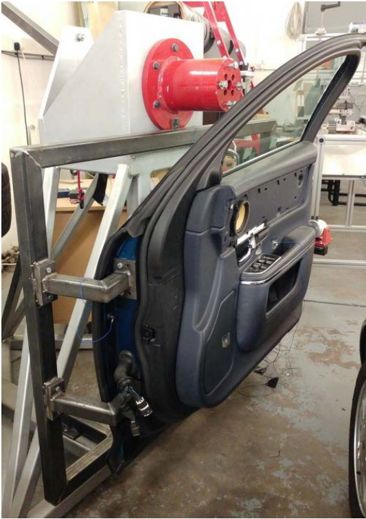
Fig. 1 – Picture of the full door assembly mounted on a heavy frame
