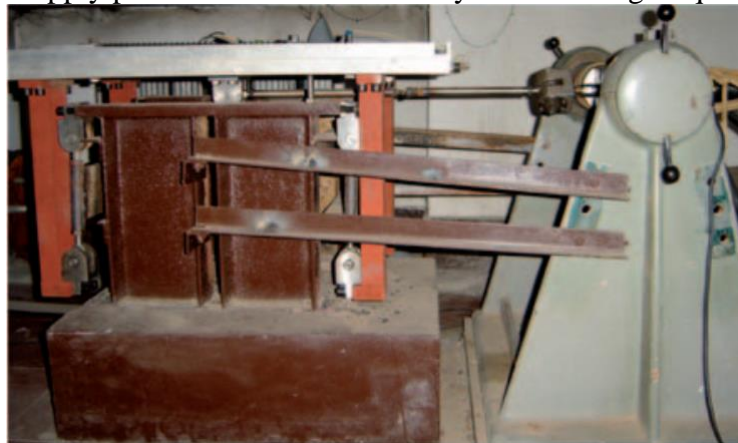
Fig. 1. The hydraulic shaking table
